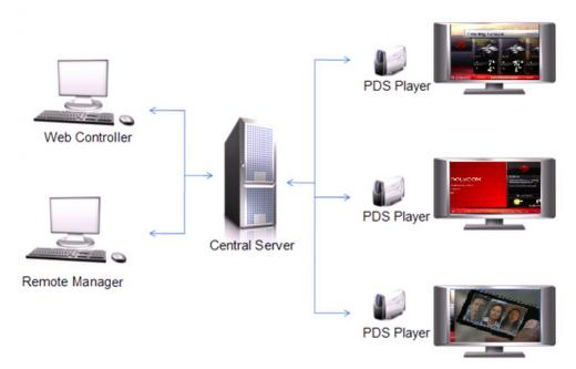
The image above presents an overview of the Polycom Digital Signage solution, depicting the overarching architecture for the various components of the solution. Content, in the form of templates, assets, and playlists, is created, assembled and managed using the Polycom Digital Signage Web Controller. Users can easily update content using the Web Controller's point-and-click interface.
